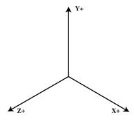
Let f be the distance to the far plane and n the distance to the near plane. Assume that r = 1, l = -1, t = 1, and b = -1. Define an isometric projection matrix that maps the world-space axes as shown in the picture, with the world-space origin being projected to x = 0 and y = 0.
